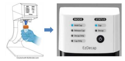
3. Press the power button for 3 seconds to select the different cycle time. The LEDs will blink when setting the cycle time.
